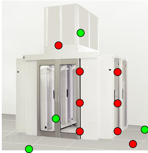
Figure 2: Representative Photograph of Hot Aisle Containment Test Installation
