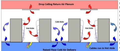
of perforated tiles. Make sure the back side of the racks on either side of the row is discharging hot air into the hot aisle. I've used configurations where the hot aisle can be from two to four feet wide, or one to two floor tiles widths. Wider
