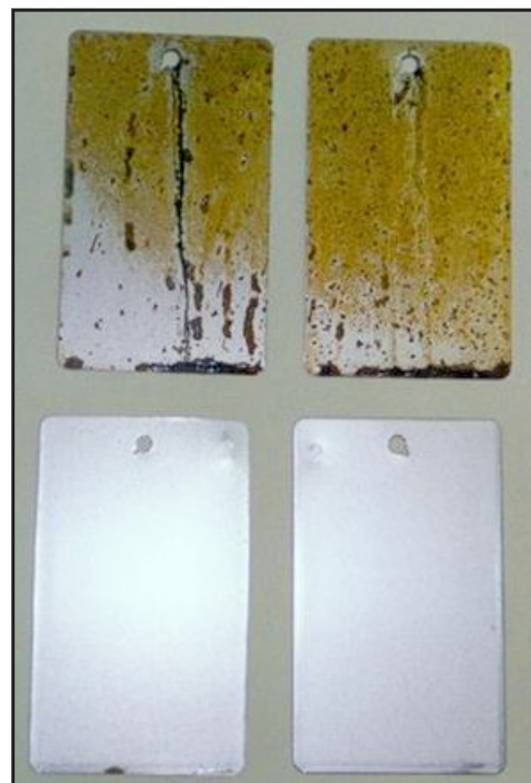
Photo of laboratory test panels. The clean panels were treated with layup chemistry. The rusty panels were not.
