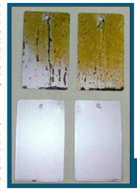
**Tower** layup treatment should be added and allowed to circulate per the direction of your water treatment provider. (Effective layup chemistry will remove both organic and iron oxide deposits, promote passivation of system metallurgies, and produce an effective and tenacious thin film barrier that will provide system corrosion protection all winter long)
